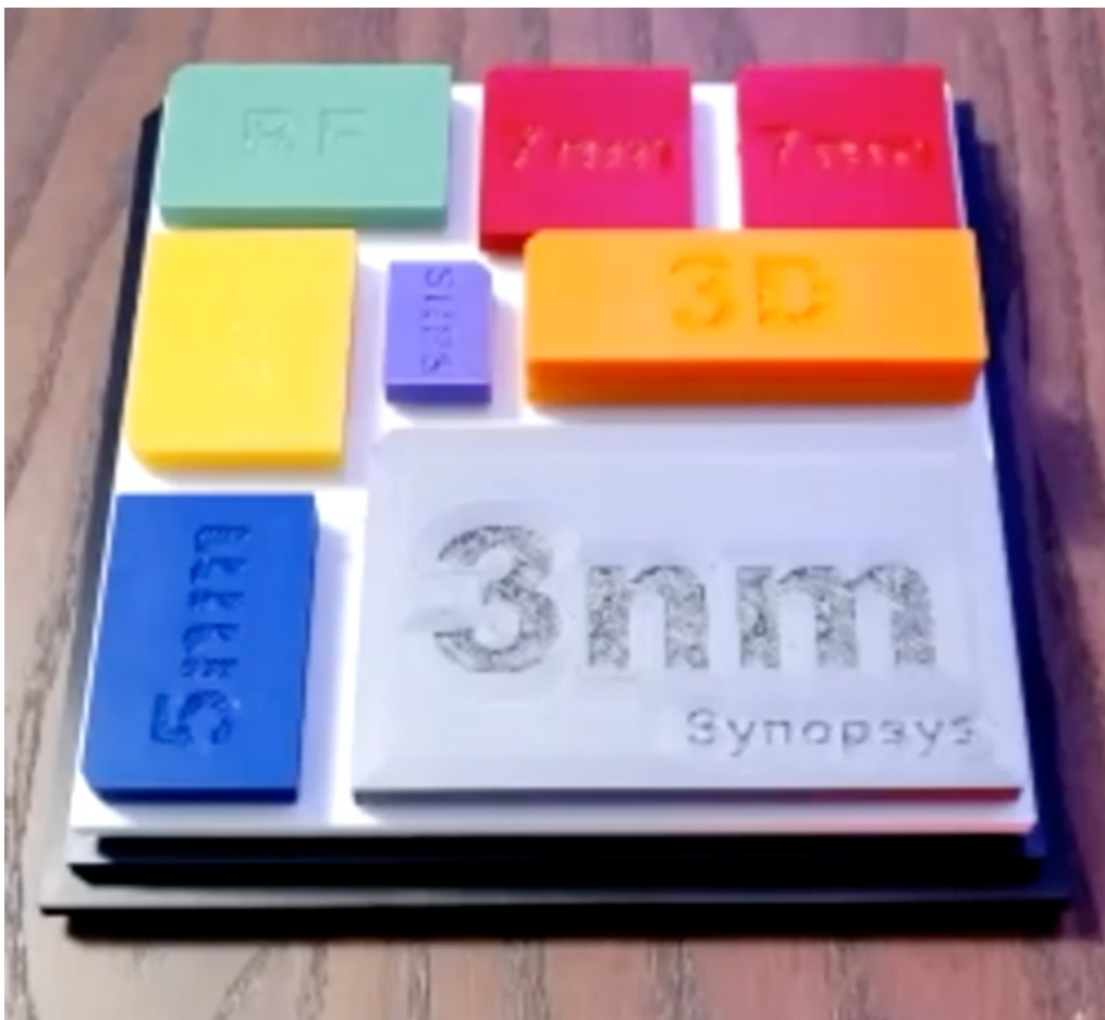
Fig. 6: A model showing a system in package consisting of chiplets from differing nodes on an interposer. One chiplet shown in orange is 3D with at least two chiplets stacked vertically. The two chiplets shown in red are identical and represent using multiple identical chiplets to scale up their function. Source: Semiconductor Engineering , 3D-printed model by Michael Posner/Synopsys
